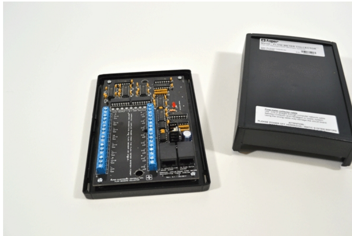
Figure 1 TM6400 Collector box
